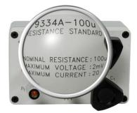
connections and can handle currents up to 100 A. **5-way beryllium copper, gold plated binding posts** are provided for measuring the voltage drop. The fifth (gold) connector is for chassis ground. Lead Set 92302 is recommended when sourcing 20 A to 100 A of current across the "C1" and "C2" connectors to avoid conducting thermal energy into the resistance element through the terminal connection.
