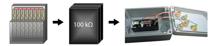
Guildline standards are the best by design and by manufacture. One key advantage of Guildline Resistance Standards is that each Resistance Value is made up from multiple resistance elements, not just a single element which is the technique used by most manufacturers.
