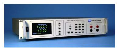
The Model 515 High Accuracy Reference Generator fills a need for a relatively low cost and practical solution for supplying a reference excitation to typical LVDT and Synchro/Resolver transducers. The Model 515 has built-in load sensing which, in effect, yields "zero" output impedance and virtually eliminates the effects of fluctuating output loads. With up to 15 Watts of output power into loads with as much as 90° of phase shift, the Model 515 is ideally suited to driving inductive loads.
