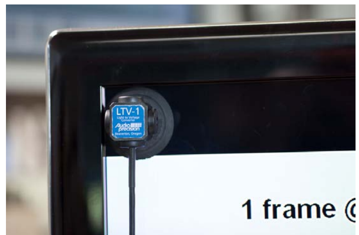
LTV-1 mounted on an LCD television monitor. The black bar at the top to the screen will flash white for sync.
